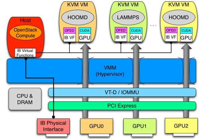
**Figure 1.** Node PCI Passthrough of GPUs and InfiniBand
