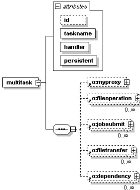
Figure 2 XML schema of multitask represents a DAG. It shows the relationship of Grid tags by defining dependency tag in GTLAB.
