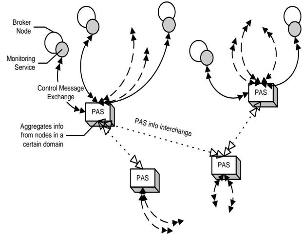
Figure 5: Multiple Performance Aggregators monitoring different domains/realms
