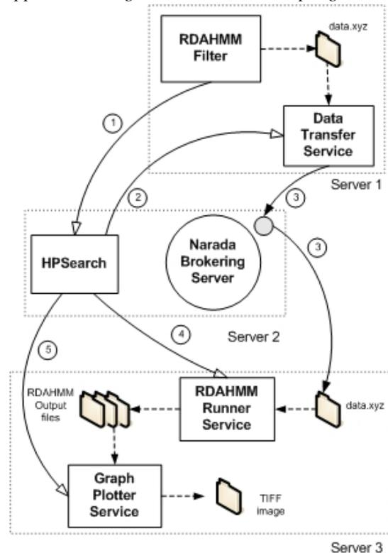
Fig. 3. System Architecture diagram for coupling RDAHMM with real-time GPS messages.
