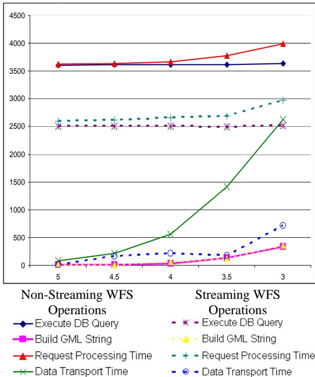
Fig. 1. Performance comparisons of the streaming and non-streaming WFS implementations showing the advantage of streaming the data over a messaging broker.
