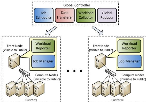
Figure 1. Hierarchical MapReduce Architecture
