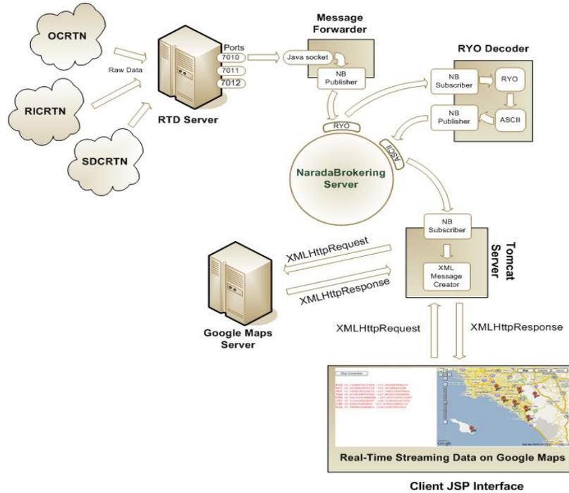
**Figure 3 Naradabrokering may be used to support filters of real-time GPS data.**
