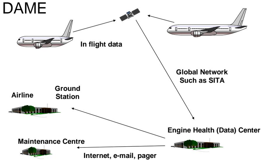
Fig. 2: Distributed Aircraft Maintenance Environment
